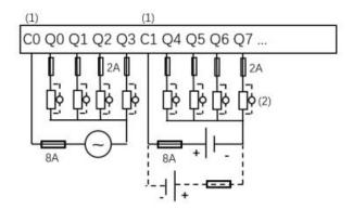
C0 和 C1 端子未在内部连接。C0 and C1 terminals are not connected internally.
