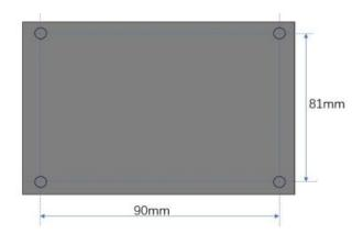
● 下图为具有 40 点 I/O 的 CPU 本体的安装孔间距 The following diagram shows the mounting holes for the 40 points I/O CPU.
